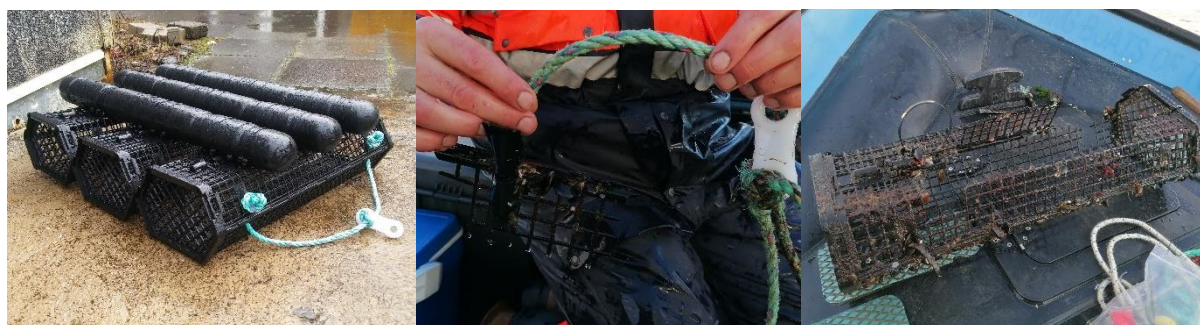
Figure 39. AP6 oyster basket. Wear and tear and storm damage in February 2024, ©SAMS.
