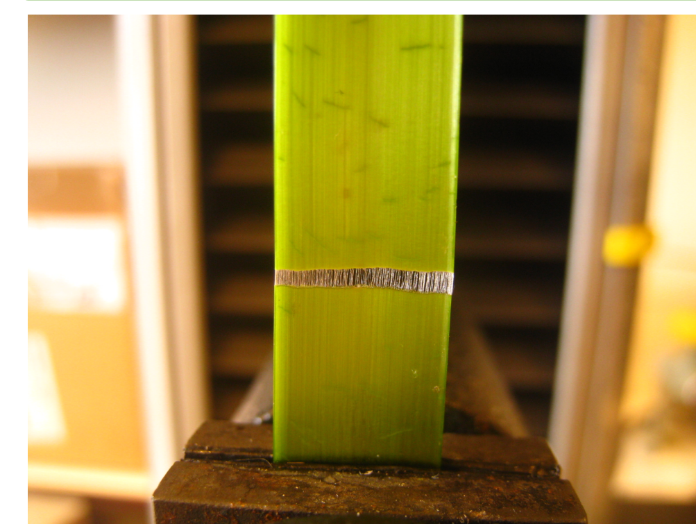
Photo 1 P. oceanica tested in a tensiometer (Instron).
