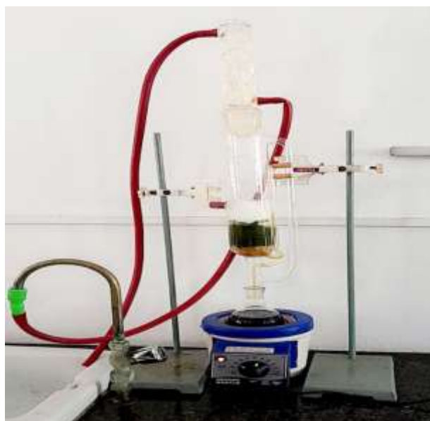
Fig 2: Preparation of plant extract using Soxhlet Apparatus.
