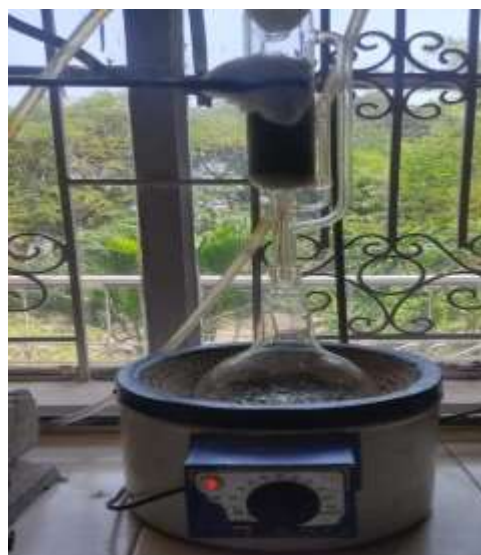
Fig.4. Continuous hot percolation method for Tylophora indica
