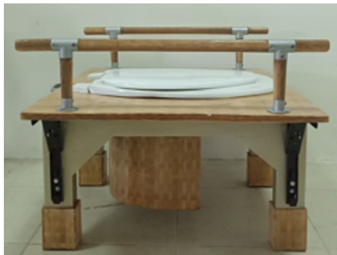
Fig. 2. The prototype produced by Universiti Muhamadiyah Yogyakarta (UMY) using the bamboo composite (Sosiati et al. 2024)
