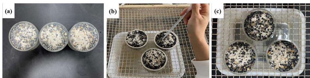
Fig 5. Preparation of the residue samples. (a) Prepared samples (b) Dripping water to saturation (c) Removing gravity water.
