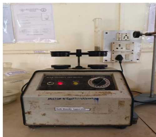
Fig 13. Tapped density tester
