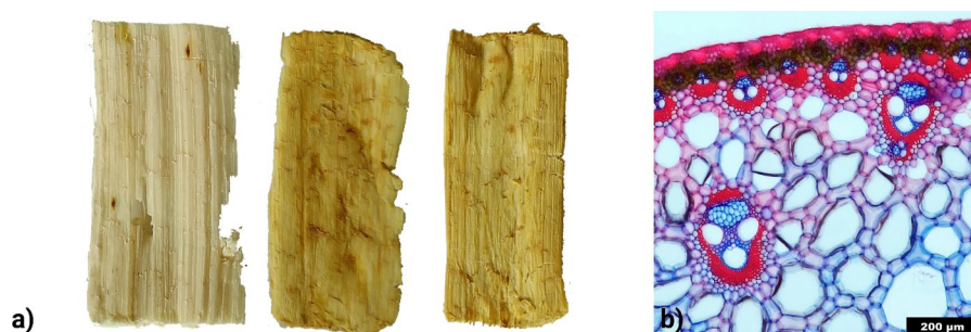
Fig. 6 Color change of papyrus pith after alkaline treatment and lignin staining a the effect of an alkaline treatment on dried papyrus pith from Qaramos, Egypt; left, untreated sample; middle, after soaking in 4% NaOH for 1 h; right, after soaking in 4% NaOH and washing until pH-neutral; the color
