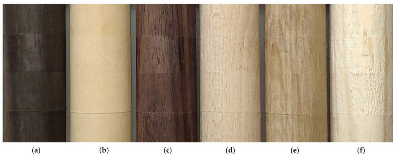
Figure 1. The wood specimens used in the tests (a) West African Ebony, Diospyros crassiflora (EB); (b) San Domingo Boxwood, Phyllostylon brasiliense (BoW); (c) Rio Rosewood, Dalbergia nigra (RW) (d) Beechwood, Fagus sylvatica (BeW); (e) Oakwood, Quercus robur (OW); (f) Pinewood, Pinus silvestris (PW).
