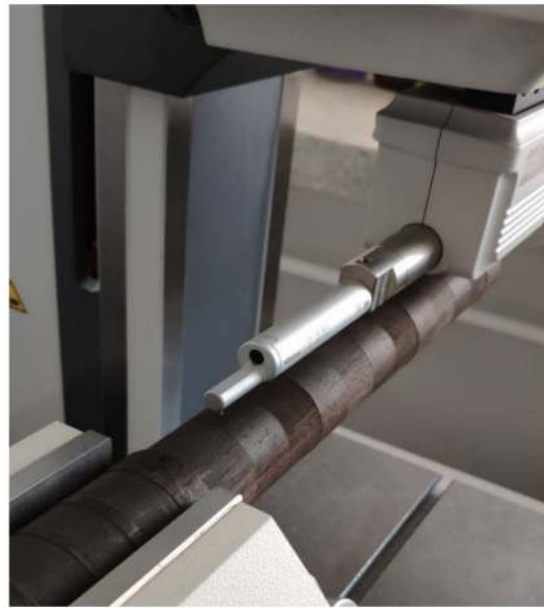
Figure 5. Placement of measurement head's needle on examined Diospyros crassiflora specimen.
