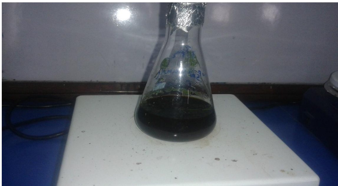
Fig 4.5 Sodium Hydroxide Pre-treatment for 15 minutes
