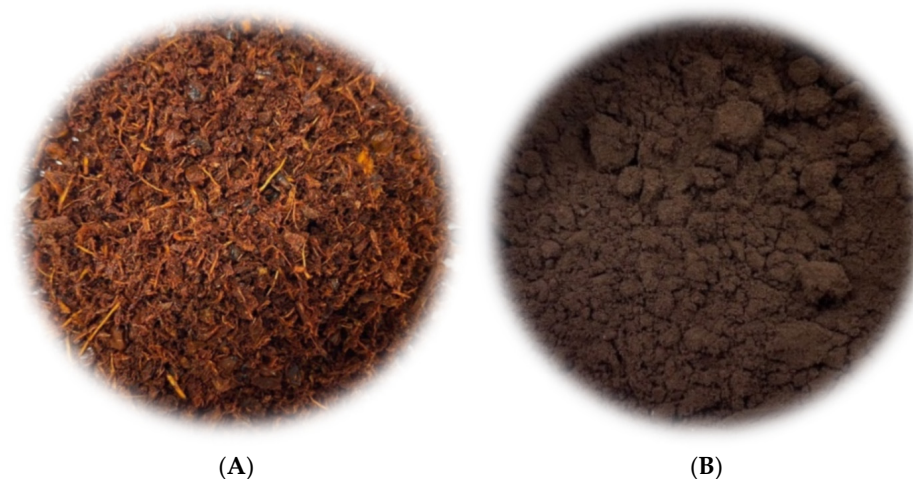
Figure 1. Visual appearance of annatto agroindustrial residue before hydrothermal treatment AW (A) and the corresponding hydrochar obtained after hydrothermal carbonization HC-AW (B).
