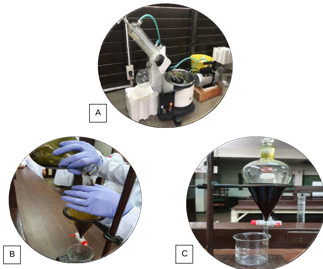
Fig. 2. S. saman extraction: (A) Rotary evaporation of macerated S. saman leaves, (B) Pouring of extract into separatory funnel, (C) Separation of polar and nonpolar compounds
