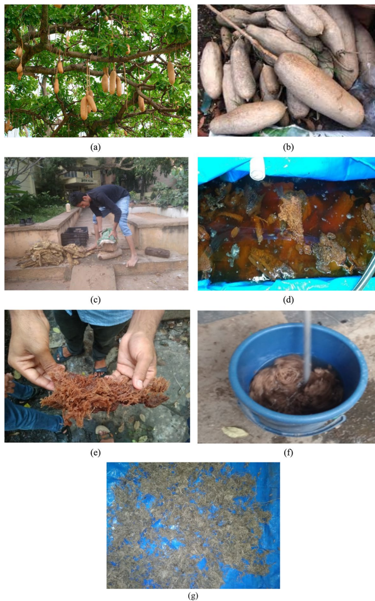
Fig. 2 a Kigelia Africana fruit, b fruits dried in sunlight for 3 days, c then fruits are crushed, d fruits are soaked in water for 3 weeks, e water retting process, f chemical treatment to remove of lignin and cellulose, g dried fibres
