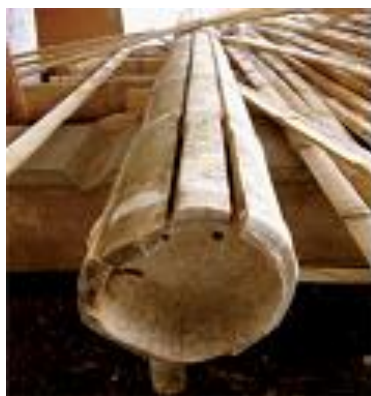
Figure 2. Initial cuts in the Bamboo GAK.
