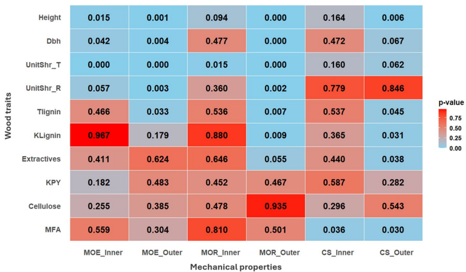
Fig. 6 Heatmap showing p-values from Pearson correlations between mechanical properties and wood traits in Eucalyptus hybrids . Color intensity reflects the level of statistical significance, with blue indicating more significant correlations (lower p-values) and red indicating less significant correlations (higher p-values). Modulus of elasticity (MOE); modulus of rupture (MOR); compressive strength (CS); diameter at breast height (DBH); unit shrinkage at tangential and radial direction (UnitShr_T and UnitShr_R); kraft pulp yield (KPY); micro fibril angle (MFA)
