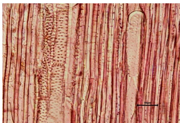
Figure 2. TLS showing alternate inter vessel pits and simple perforation in vessel.
