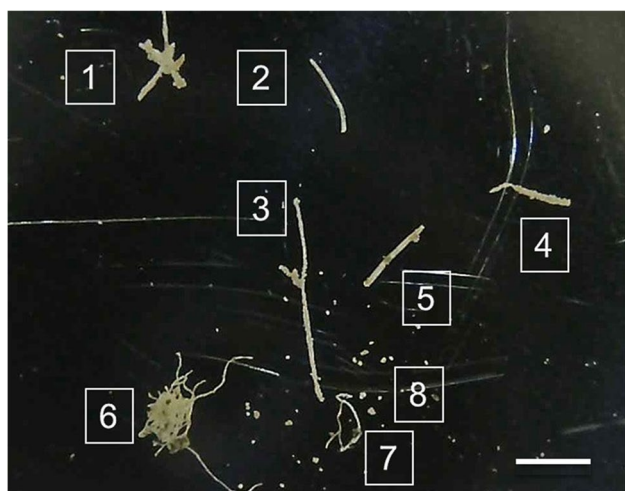
Fig. 13 Microscope image of the fibres and particles analysed with Raman spectroscopy: (1) rough, irregular fibre cluster; (2) thin, smooth fibre; (3) thin, rough fibre; (4) irregular, rough fibre; (5) thick, smooth fibre; (6) thin fibre cluster; (7) thin, irregular fibre; (8) irregular, shiny particles. Scale bar: 1 mm
