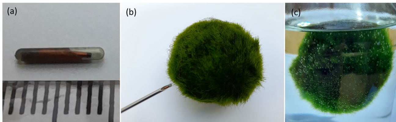
Fig. 8 Photographs of (a) an RFID microchip encapsulated in a bioglass capsule, (b) inserting the capsule into a Marimo with an applicator, (c) Marimo floating with an RFID tag in the centre
