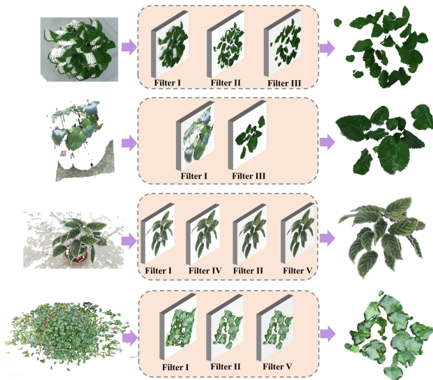
FIGURE 3. Concatenations of filters used for preprocessing the point clouds of four types of sample plants, respectively. The first row shows the filters used for processing the point cloud of Epipremnum aureum sample plant, including Filter I, Filter II, and Filter III. The second row demonstrates the filters used for processing the point cloud of Monstera deliciosa sample plant. The third row shows the filters for the point cloud of Calathea makoyana sample plant. The fourth row shows the concatenation of filters for processing the point cloud of Hedera nepalensis sample plant.
