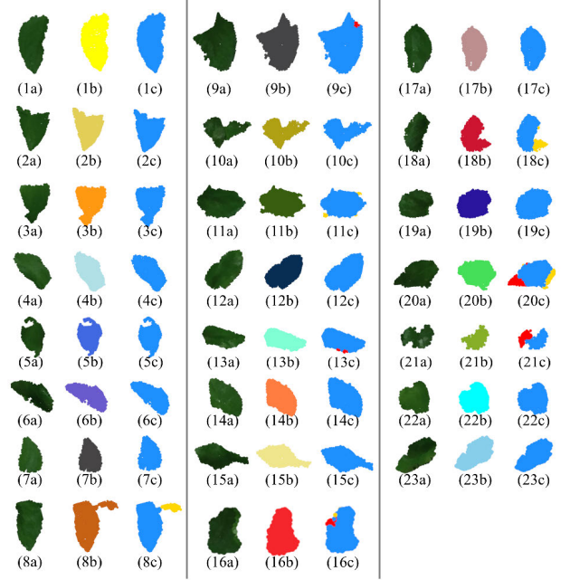
FIGURE 11. The color labeled point-level quantitative measures for all leaves in the Epipremnum aureum point cloud. The columns that with label “(a)” contain the ground truth of individual leaves rendered by real colors. The columns that with label “(b)” show results of the proposed segmentation algorithm, and each segmented leaf is painted with a different color; the columns that with label “(c)” demonstrate color labeled point-level measures in the same way as Figure 10(c).
