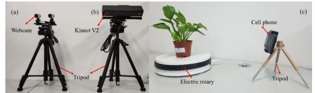
FIGURE 1. Three types of imaging platforms used in this research. (a) shows the binocular stereo vision platform containing two high-definition webcams; (b) shows the platform of the Kinect V2 sensor mounted on a tripod; (c) shows a multi-view stereo vision platform containing a cell phone, an electric turntable, and the VisualSFM software.
