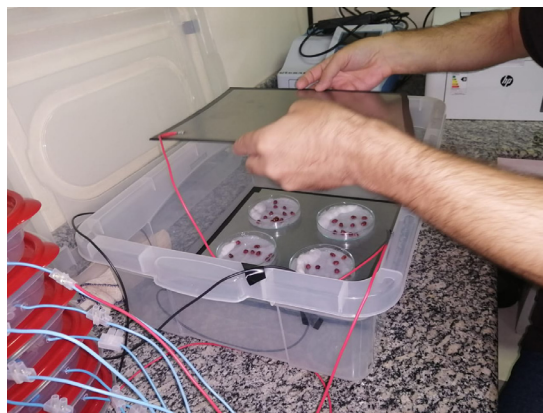
Fig. 3. Seed samples in Petri dishes on wet filter paper between stainless steel plates.
