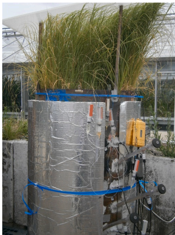
Fig. 1. Photo of a soil core with Rhodes grass after irrigation with 3200 mm coal seam (CS) water and 2200 mm deionised (DI) water (left), and the schematic layout (right) of the soil core.
