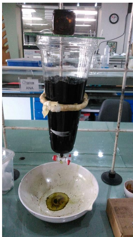
Figure 2: Percolation setup showing the interaction between the botanical matrix and the extraction solvent.
