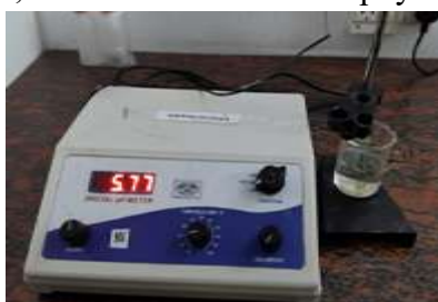
Fig No.8: pH meter showing value for F1
