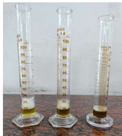
Fig No. 12: Foam height of F1, F2 and F3
