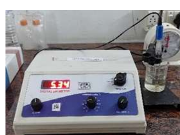
Fig No.10: pH meter showing value for F3
