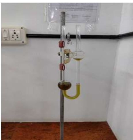
Fig No.11: Ostwald viscometer showing viscosity measurement
