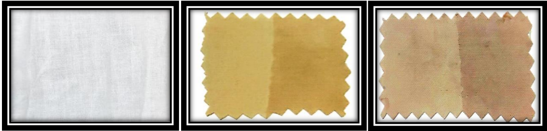
(a) (b) (c) (d) (e) Figure 13: Discharged cotton fabrics using taro corms extract at the optimum time (a) blank fabric (b) Discharged Guava dyed fabric (c) Guava dyed fabric (d) Discharged Ficus dyed fabric (e) Ficus dyed fabric
