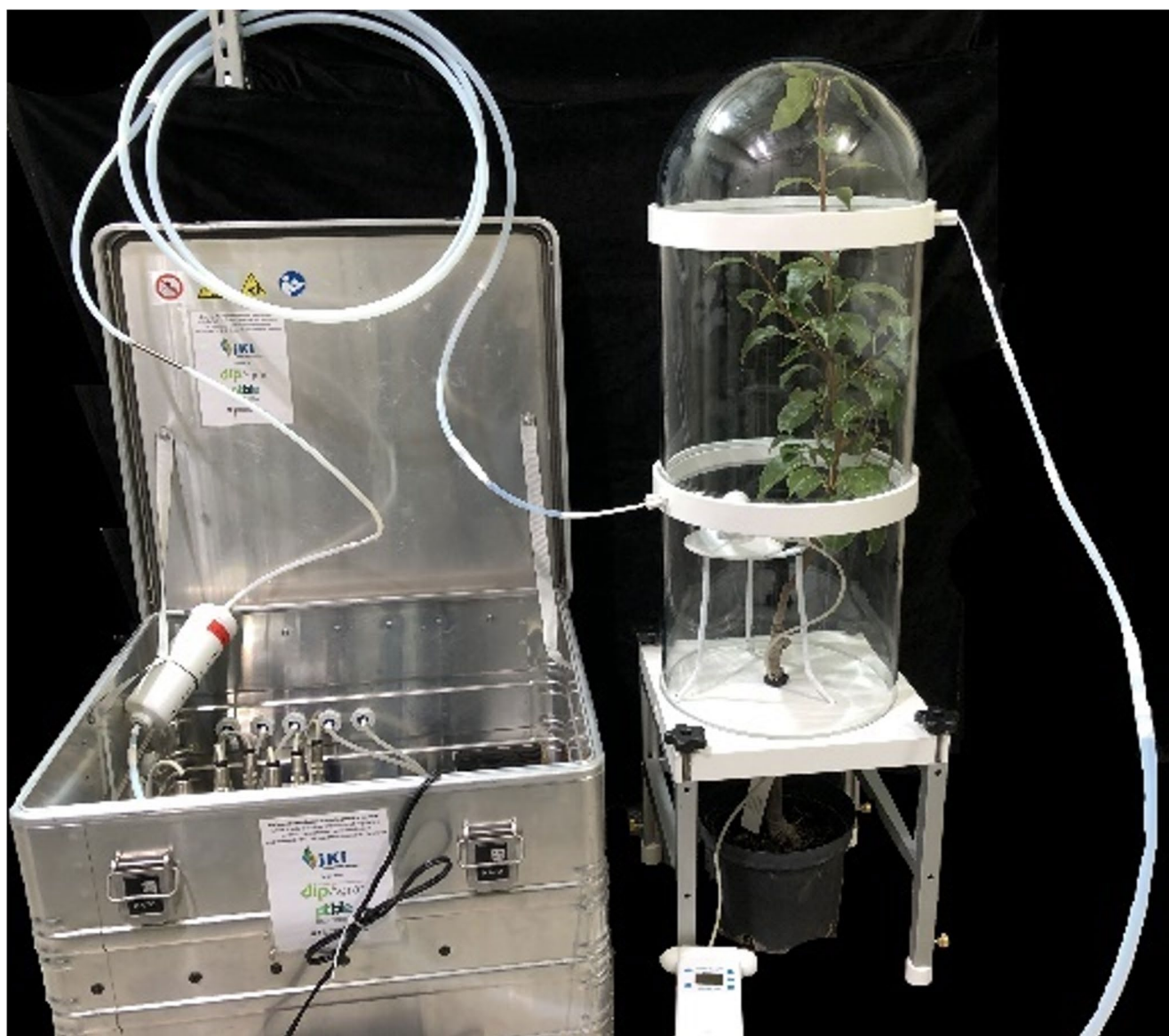
Fig. 2 Headspace sampling set up. Pear tree ( Pyrus communis ) placed in a sectional adjustable high volatile glass collection chamber connected via PTFE tubing to a mobile headspace sampling device. An
