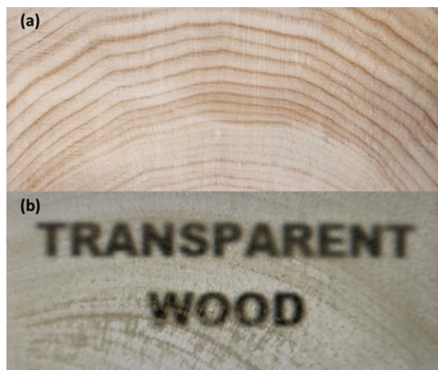
Fig. 1 Investigated samples of pristine basswood a and prepared epoxy-based transparent wood b
