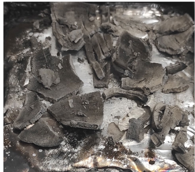
Fig. 8 Char residue of transparent wood after being loaded by 20 kW m -2 heat flux during 1,800 s
