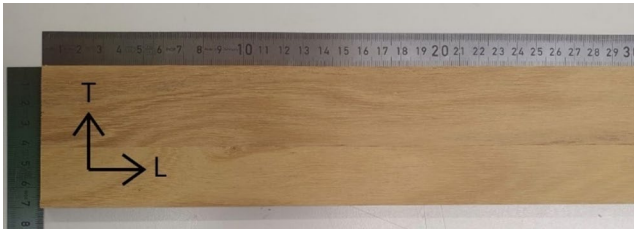
Fig. 5 Three-ply LVL-board in longitudinal-tangential (LT-) plane for the determination of \mu_{LT} ; dimensions in cm
