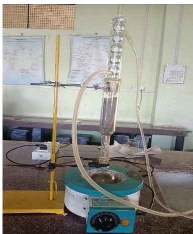
Figure 1: Extraction of oil from nigella sativa seeds using soxhlet apparatus.
