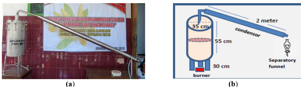
Figure 1. (a) Real picture of distillation reactor; (b) Schematic representation of distillation reactor for extraction of cananga oil
