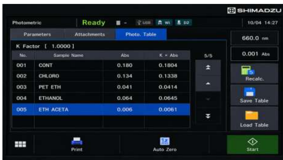
Fig.3.12 UV-Visible Spectrophotometric Measurement of Absorbance of different extracts at 660 nm in Protein Denaturation Assay
