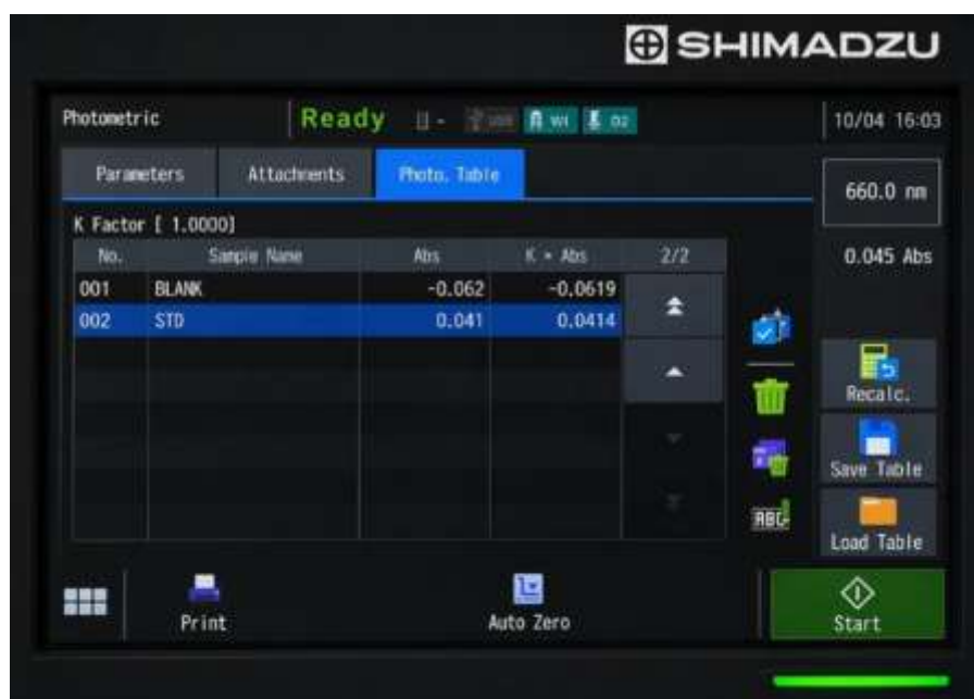
Fig.3.11 UV-Visible Spectrophotometric Measurement of Absorbance at 660 nm in Protein denaturation Assay
