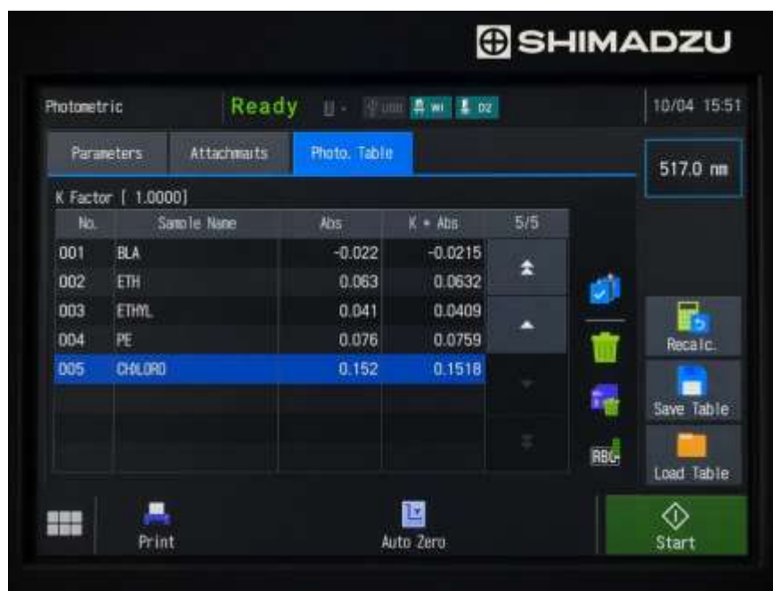
Fig.3.9 UV-Visible Spectrophotometric Measurement of Absorbance of different extract at 517 nm in DPPH assay
