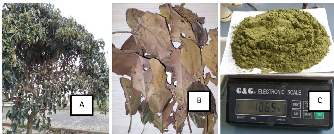
Fig. 1 Stages of biosorbent development from Cordia africana leaves: Cordia africana tree (A), dried Cordia africana leaves (B), and ground ready-made biosorbent (C)
