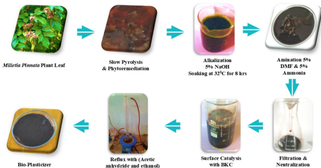
Fig. 1 Extraction of bio-plasticizers from Millettia pinnata plant leaf
