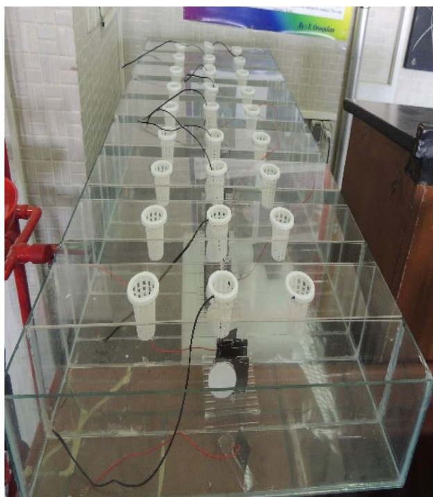
Fig. 2 Initial structure of the plant microbial fuel cell evaluated in this study
