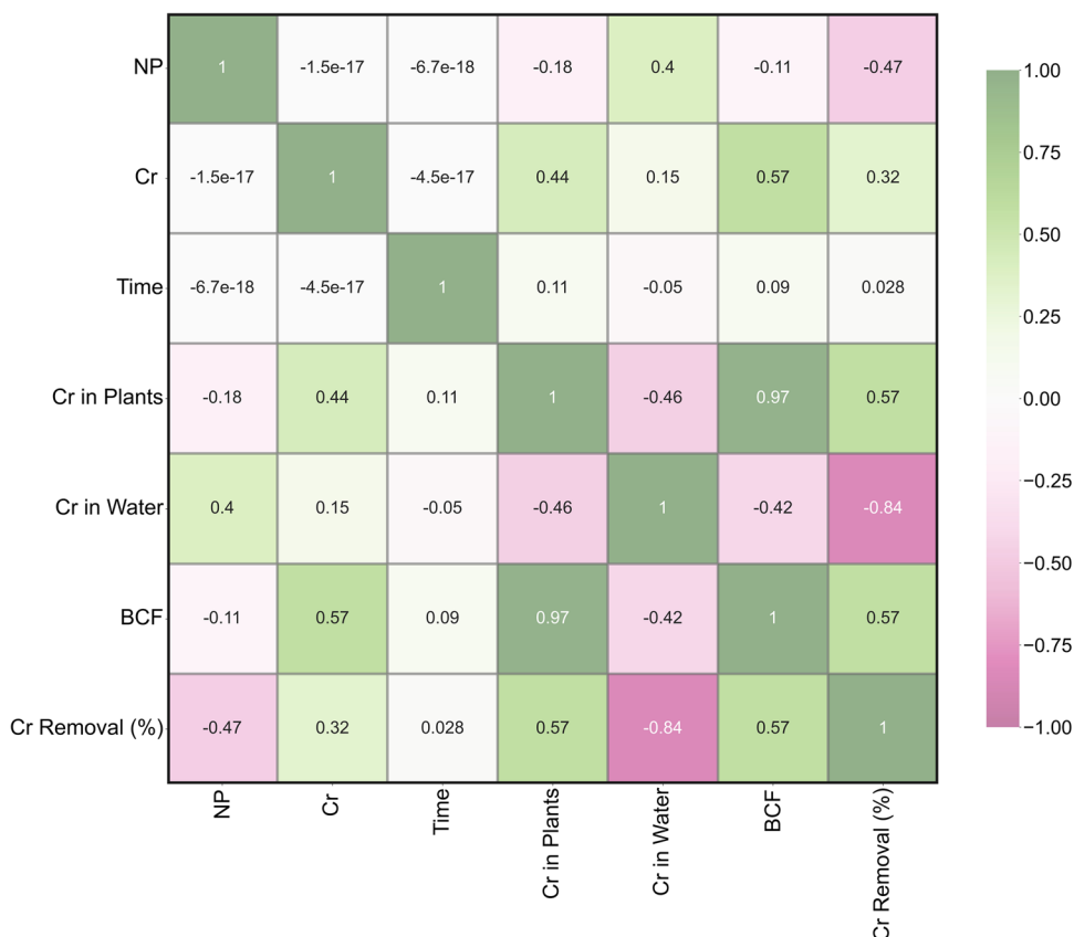
Fig. 5 Correlation heatmap between input and output variables for nano-phytoremediation of Cr
