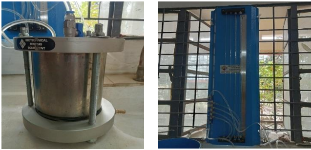
Figure 8. Permeability testing of soil specimen
