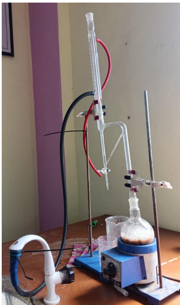
Fig. No. 05: Assembly of Ginger Extraction using Cleveanger apparatus.
