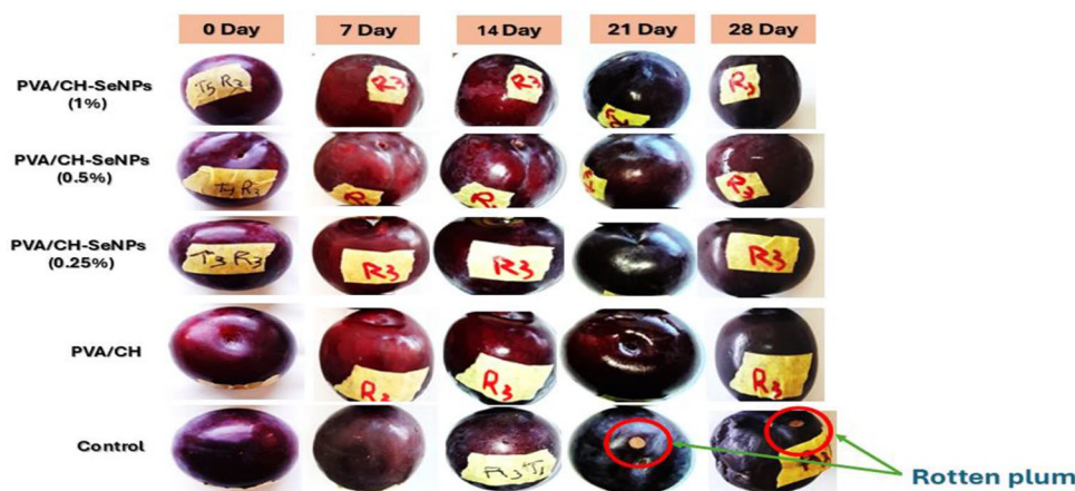
Fig. 13 Impact of PVA/CH and PVA/CH-SeNPs films on enhancing storability of Hollywood plum during cold storage conditions (at 0 \pm 2^\circ\text{C} and 90 \pm 5\% RH)
