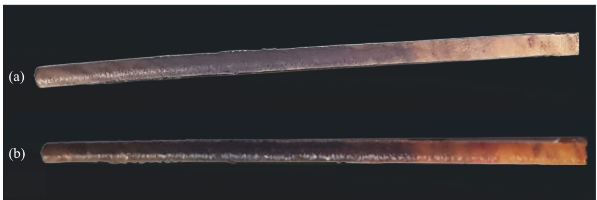
Fig. 2 Identification of sapwood and heartwood depths using an indicator dye (a) core sample after extraction from the tree trunk (b) colour change observed after applying methyl orange indicator dye
