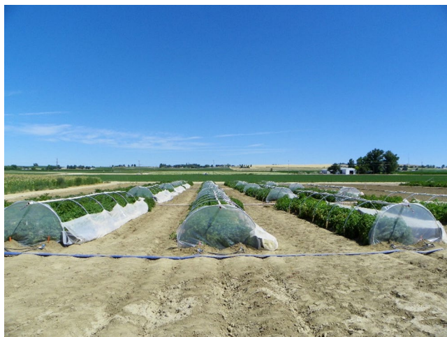
Fig. 1 Enclosures made from clear plastic, PVC pipe and metal hoops used to cover both smoke and non-exposed plots. The plastic and shade cloth along the right side was rolled over each enclosure before the start of the daily exposure period (6 am) and then removed when the exposure period ended (9 am)
