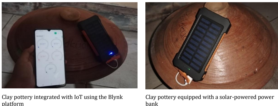
Fig. 9. Innovative Pottery System with Solar-powered IoT Integration.
