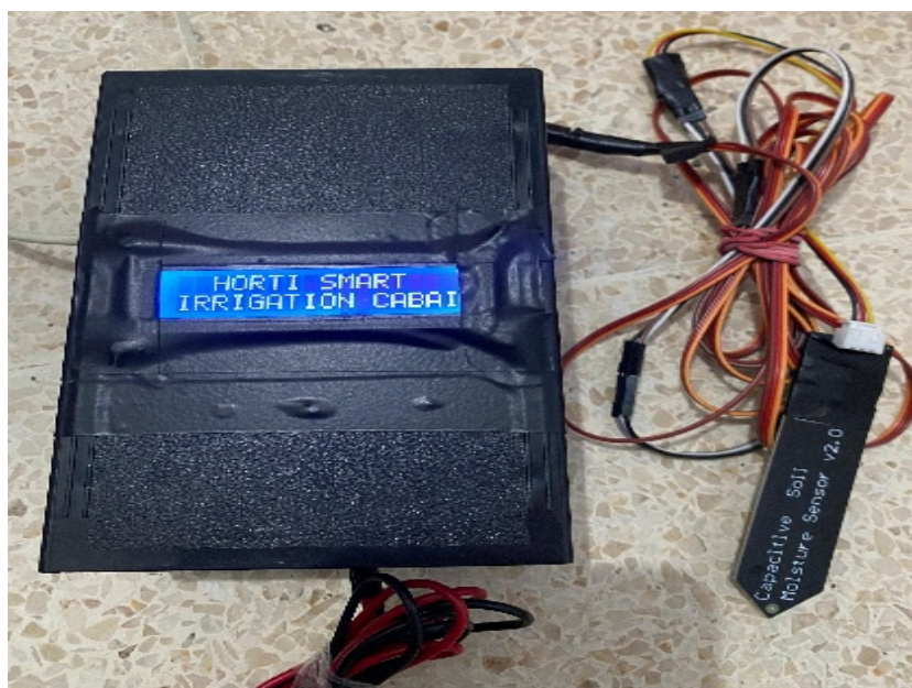
Figure 3. Prototype automatic irrigation equipment size (14 x 8.2 x 3.8) cm
