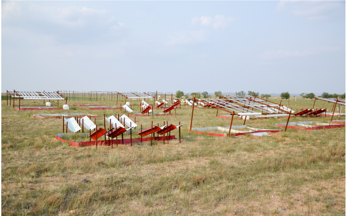
Photo 2. The experimental facility in field. We applied rainout shelters to achieve 50% and 25% precipitation reduction by changing the number of V-shaped acrylic strips. A steel pipe frame was used to support the V-shaped acrylic bands (92% light transmittance). For the precipitation addition treatments, four and eight V-shaped steel sheets were uniformly located outside the plots for the 25% and 50% addition treatments, respectively. Photo credit: Quanhui Ma.
