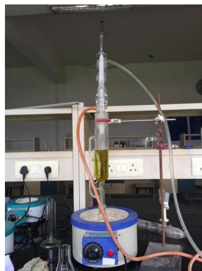
Figure 2: Methanolic extraction of Smilax China in Soxhlet apparatus.
