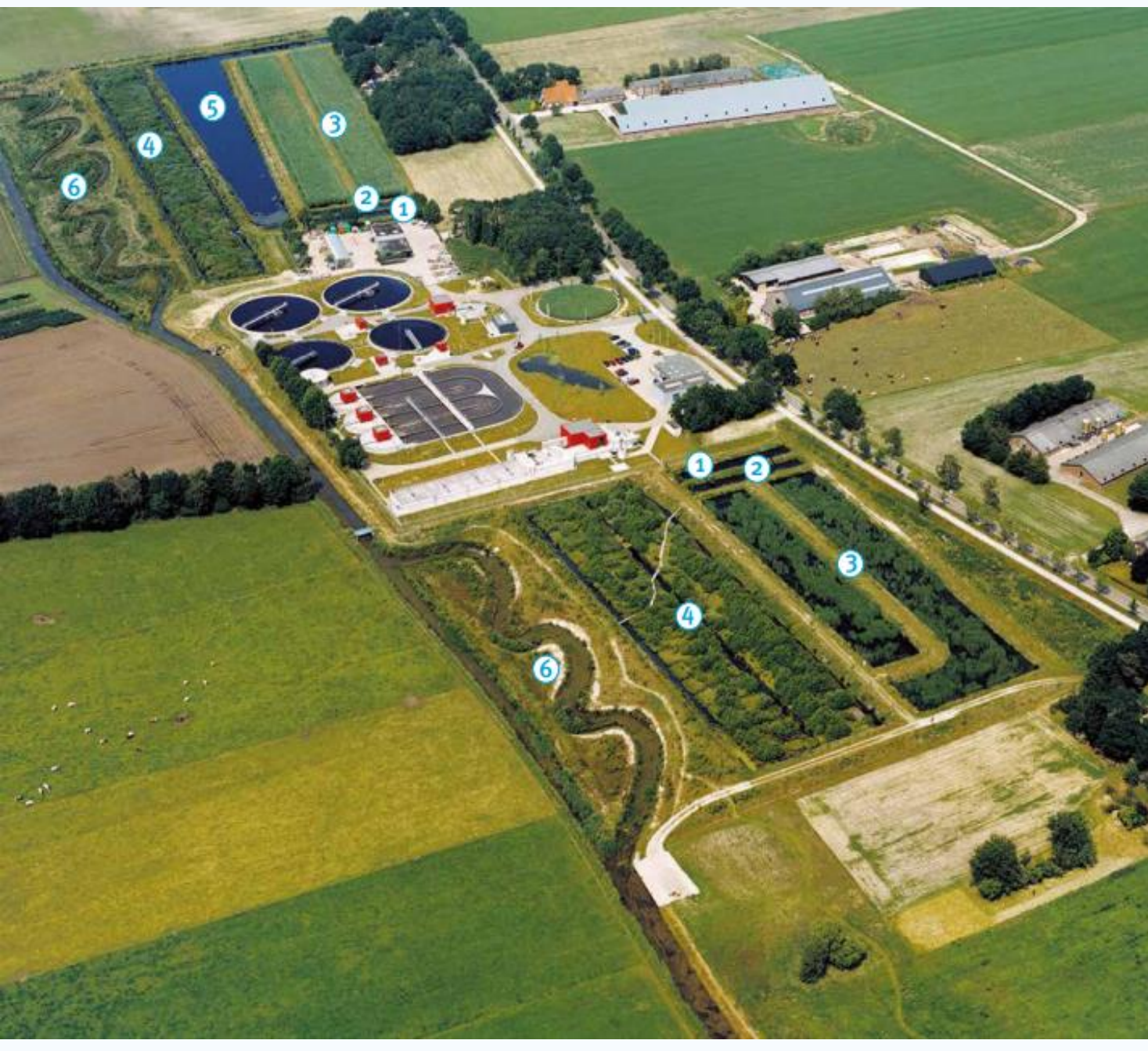
Fig. 1. Constructed wetlands for the post-treatment of WWTP effluent: 1) Bufferditch; 2) Distribution ditch; 3) Surface flow constructed wetland with common reed; 4) Swamp Forest; 5) Surface flow constructed wetland without plants; 6) Stream restoration.
