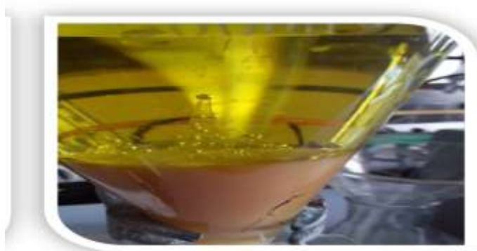
Photo 3: Two phases of Eryngium bourgatii ethanol-hexane extract (oily and aqueous)
