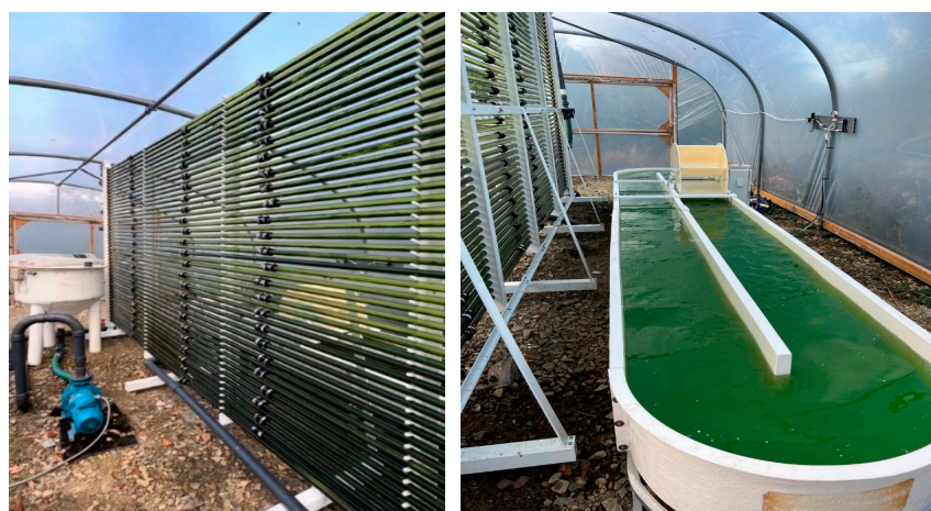
Figure 1. Horizontal tubular photobioreactor (400 L capacity (left)) and raceway (1000 L capacity (right)) installed inside of a polytunnel. Both systems received CO 2 waste gas from the brewery on site (source: A. Silkina, personal photos).
