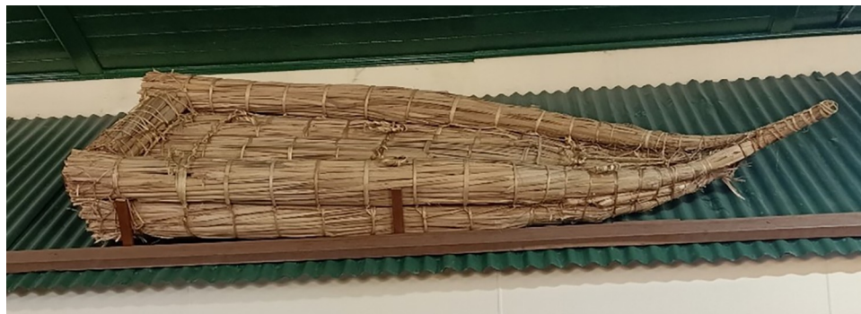
Fig 4. A mōhiki constructed from raupō stems, Kurow museum (Aotearoa New Zealand). Photo: Rewi Newnham.
