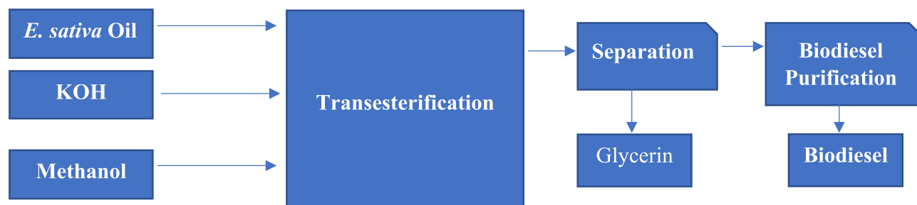
Fig. 2. Schematic flow chart of transesterification reaction procedure.
