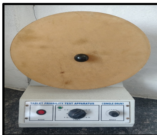
Fig no. 6: Friability test apparatus
