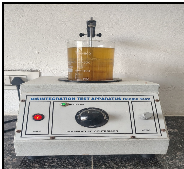
Fig no. 9 : Disintegration Test Apparatus
