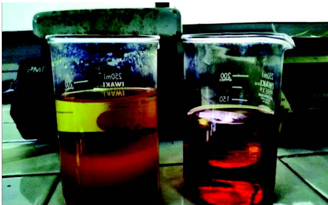
Figure 10. Fatty acid metil ester (FAME): (a). esterification (b) biodiesel.
