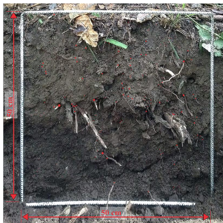
Figure 3. Trench section area ( 50 \times 50 cm) of a chestnut tree with root sections highlighted.
